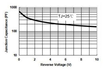
Fig.1-Typical Junction Capacitance
