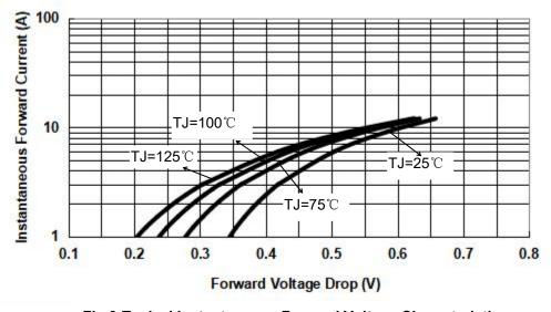
Fig.3-Typical Instantaneous Forward Voltage Characteristics
